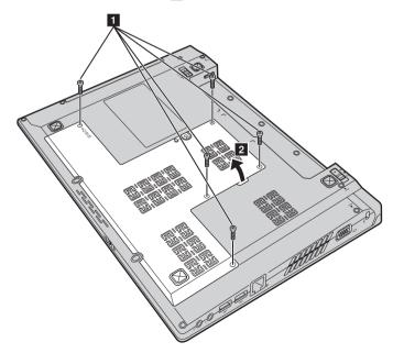
(a) If two DDR3 SDRAMs are already installed in the memory slot, remove one of them to make room for the new one by pressing out on the latches on both edges of the socket at the same time. Be sure to save the old DDR3 SDRAM for future use.
