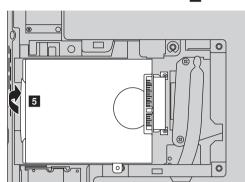
Take out the hard disk drive secured in a metal frame 5.
